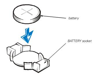
Figure 8-15. System Battery and Battery Socket
